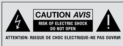
CAUTION: To prevent the risk of electric shock, do not remove cover (or back plate). There are no user serviceable parts inside. Refer servicing to qualified service personnel.
